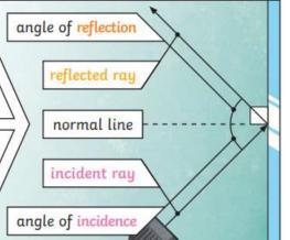
We need light to be able to see things. Light waves travel out from sources of light in straight lines. These lines are often called rays or beams of light.
